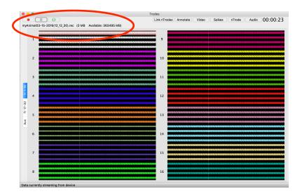
Start streaming data (see above), and then select **File->Record** to start saving data. Alternatively, you can press the record button at the top of the window. You can pause recording at any time— this does not close the file but simply stops logging. When the record button is pressed, logging continues (with a gap of data in between).
