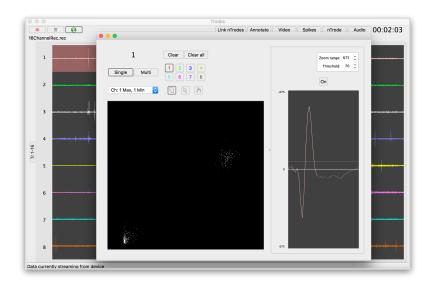
Select the 'Link nTrodes' button to link changes across nTrodes. Then, press the 'nTrode' button. You'll notice that bandpass filters are currently being applied to all channels (signified with the check mark in the spike filter section). Uncheck this, and the filters will be deactivated and you will see lower frequency signatures in the traces.
